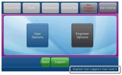
Engineer User Logged in User Level 3 times out in less than 30 seconds and returns to Key Level 2 when controls of the touch-panel-display are not operated
