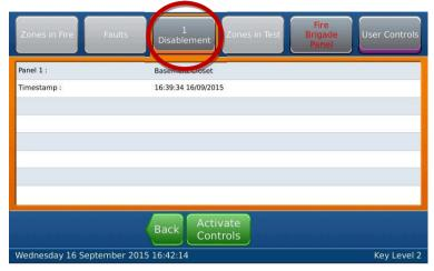
5 Press Enable or Enable All to re-enable all sounders on the fire control panel.
