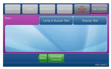
Press the Lamp & Buzzer Test button to operate the internal buzzer and light all LEDs on the fascia of the fire control panel. Press the Display Test button to provide a series of blank raster colours on the touch-panel-display.
